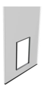
Due to technical reasons the glass panel must be chosen in a way that the spacing distance to the outer edge of the element is at least 5 cm circular (according to the glass manufacturer for stability reasons).
