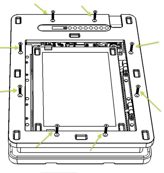
2. Lift the inner frame (part with the display) carefully with an upward movement.
