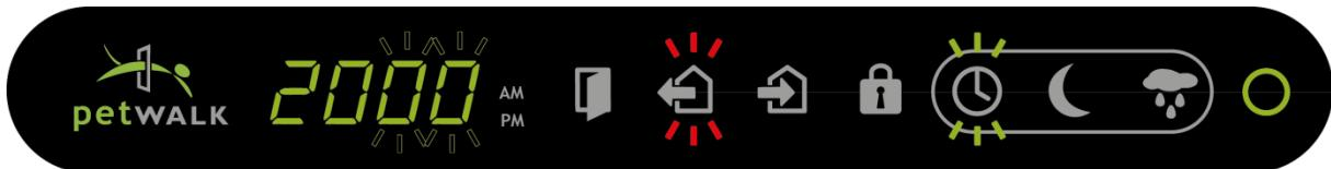
After setting times as desired, confirm the setting of the exit period with the **OK** button. Now the time span, when your pets are allowed to leave your home, is stored and you are back to the setup mode. You can leave the setup mode by pressing the **OK** button or by pressing the **Setup** button or by pressing the **Operating Mode** button.
