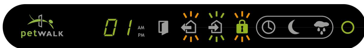
If pressing the *Entrance Control* and *Exit Control* button, the colour of the corresponding screen fields will change.
