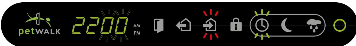
If this period is adjusted as desired, confirm the settings with **OK** . Now the time period, in which your pets can come back into the house, is stored and you are in setup mode again. You can exit by pressing the **OK** button or by pressing the **Setup** button or by pressing the **Operating Mode** .
