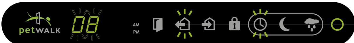
After setting the correct hour, confirm it with the *OK*
