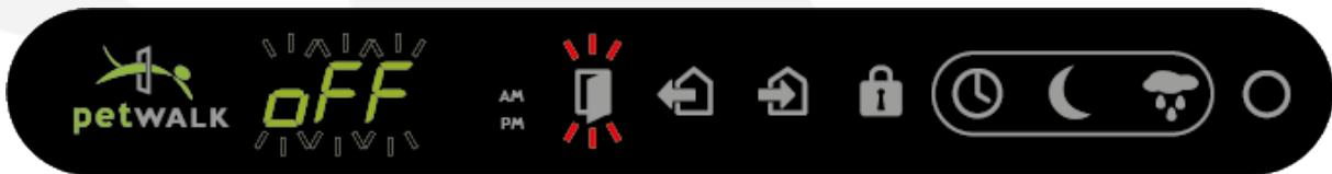
This is the factory default, where the door-in-door mode is off. Now you can switch to the desired mode by using the Up and Down buttons. If using a door contact sold by Petwalk, you must switch to normally open "nope" on display.
