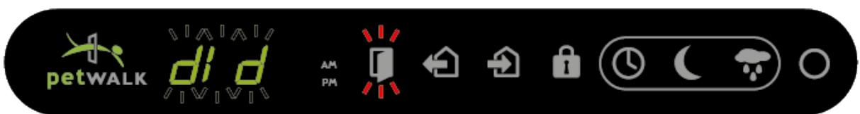
By pressing the *OK* button, you confirm the door-in-door mode. The display shows "OFF".
