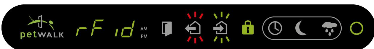
In this example it means that RFID control will be only active for the outside once Access Control is activated. On the inside the door will operate on movement control.
