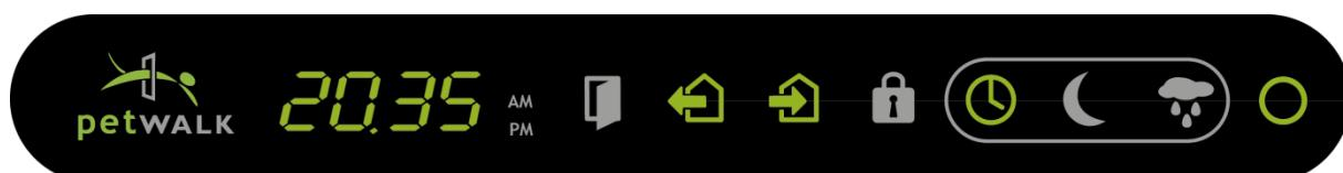
The petWALK pet door is now controlled by motion detection. If the current time is in the selected time window, the symbol turns green. If the current time is outside the time window, the symbol turns red.
