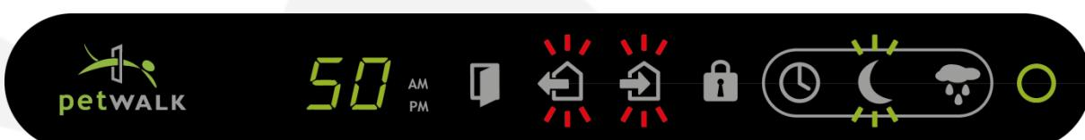
In addition to the preset dawn value (50), the symbols *Entrance Control* and *Exit Control* flash red. This means that when day light gets below this level both exit and entry is prohibited. If the symbol *Dawn Control* flashes green, the petWALK pet door is still in setting mode.
