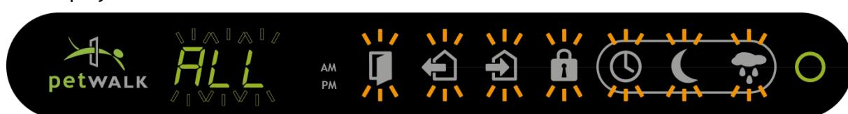
By using the *Up* and *Down* buttons you can scroll down in the settings menu until "dld" appears.
