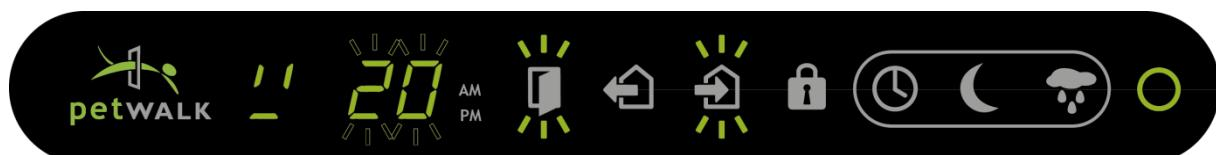
This state is signalled by a flashing *Entrance Control* symbol. You can now perform your desired change in the same way as for the exit control.
