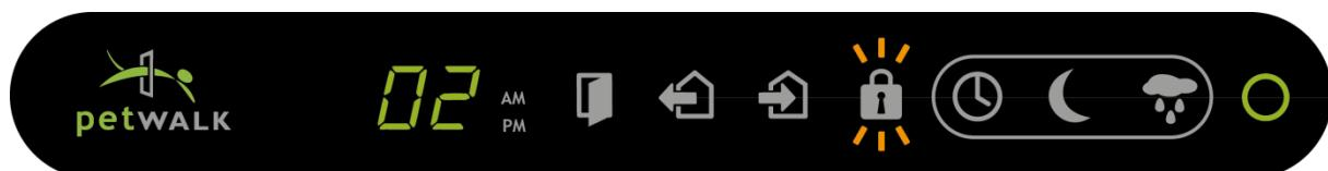
If you press the *OK*
