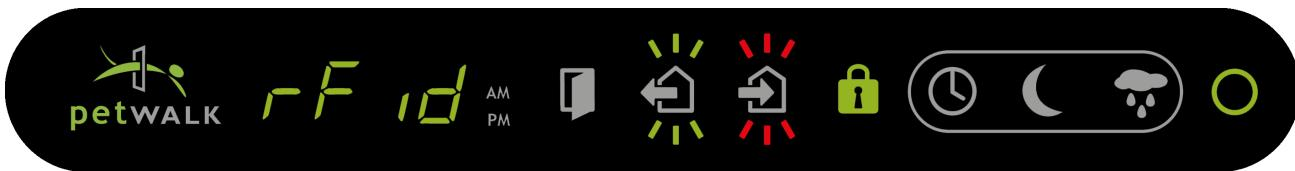
This setup means that RFID access control only works on the inside. On the outside the door opens by movement sensor.
